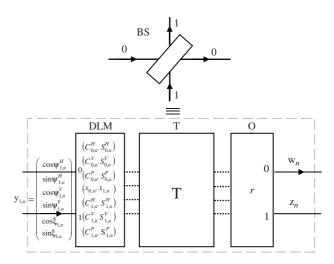
**Fig. 2.** Diagram of a DLM-based processing unit that performs an event-based simulation of a beam splitter (BS). The processing unit consists of three stages: An input stage (DLM), a transformation stage (T) and an output stage (O). The solid lines represent the input and output channels of the BS. The presence of a message is indicated by an arrow on the corresponding channel line. The dashed lines indicate the data flow within the BS. The transformation matrix **T** is given in Eq. (15).
